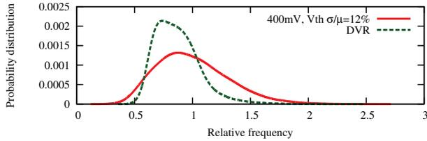
Fig. 4: Core-to-core frequency variation for DVR versus SVR. Data points are normalized to SVR die mean.
