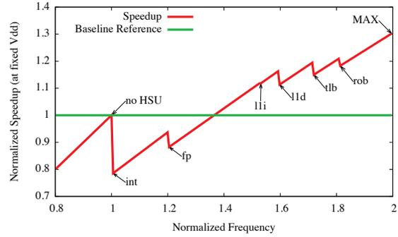
Fig. 1: Frequency vs. average speedup for a core with HSU running SPEC2000 benchmarks. Performance drops when a unit’s frequency is dropped to half-speed, but core frequency can then be increased, offsetting the the loss.
