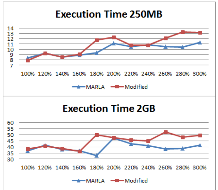
Fig. 7. Here the number of splits as a percentage of nodes in the cluster is on the X-axis, with execution time in seconds on the Y-axis. The results for MARLA and our framework with a boundary of 110°C are displayed.
